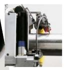
TILT-AVC standard. Allows the torch to be pivoted for socket/fillet welding applications, maintaining the arc length correction motion along the tungsten electrode axis [tilt-torch bracket also provided standard].
